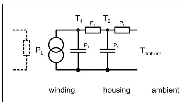
**Schematic drawing of the model of the thermal behaviour:** The power loss  $P_L$  in the armature flows through the housing to the ambient. The temperatures  $T_1$  and  $T_2$  represent the temperatures of armature and housing. The parameters  $P_1$  to  $P_4$  depend on the physical properties.
