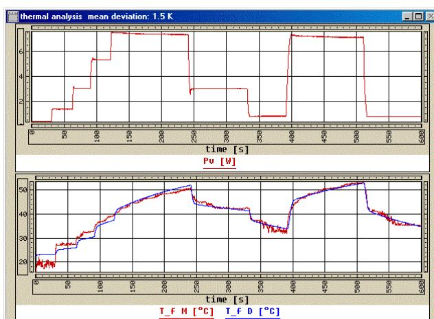
**Identification:** The upper diagram shows the power loss heating the motor. The lower diagram shows the measured temperature (red) and the estimated temperature (blue), calculated with the identified set of parameters.
